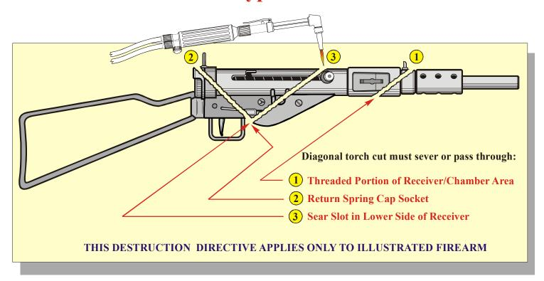
The purpose of this procedure is to destroy the receiver or frame in a manner that will prevent its function and future use as a firearm. A proper method of destroying this firearm is to cut the receiver into separate pieces as follows:
