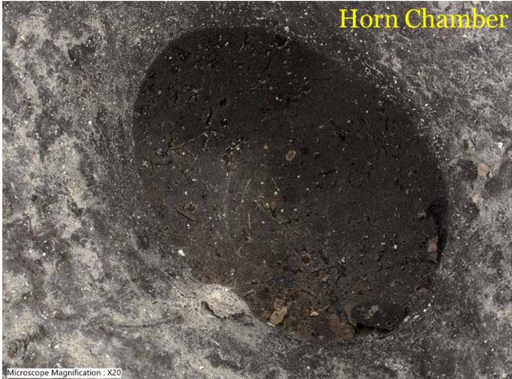
Figure 6. Example of a smoke alarm with thermal damage sufficient to alter observable indicators. Note the deformation and discoloration on the horn chamber.
