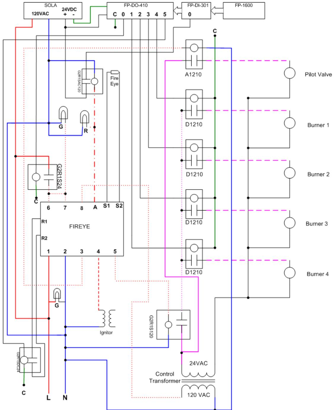
Figure 13. Wiring Diagram for Tube Burner Electrical Box
