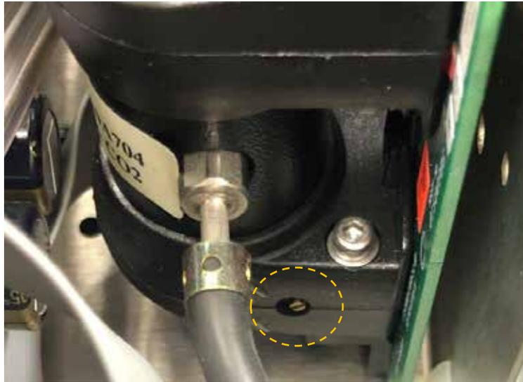
**Figure A3. CO<sub>2</sub> Cell Coarse Zero Potentiometer**
