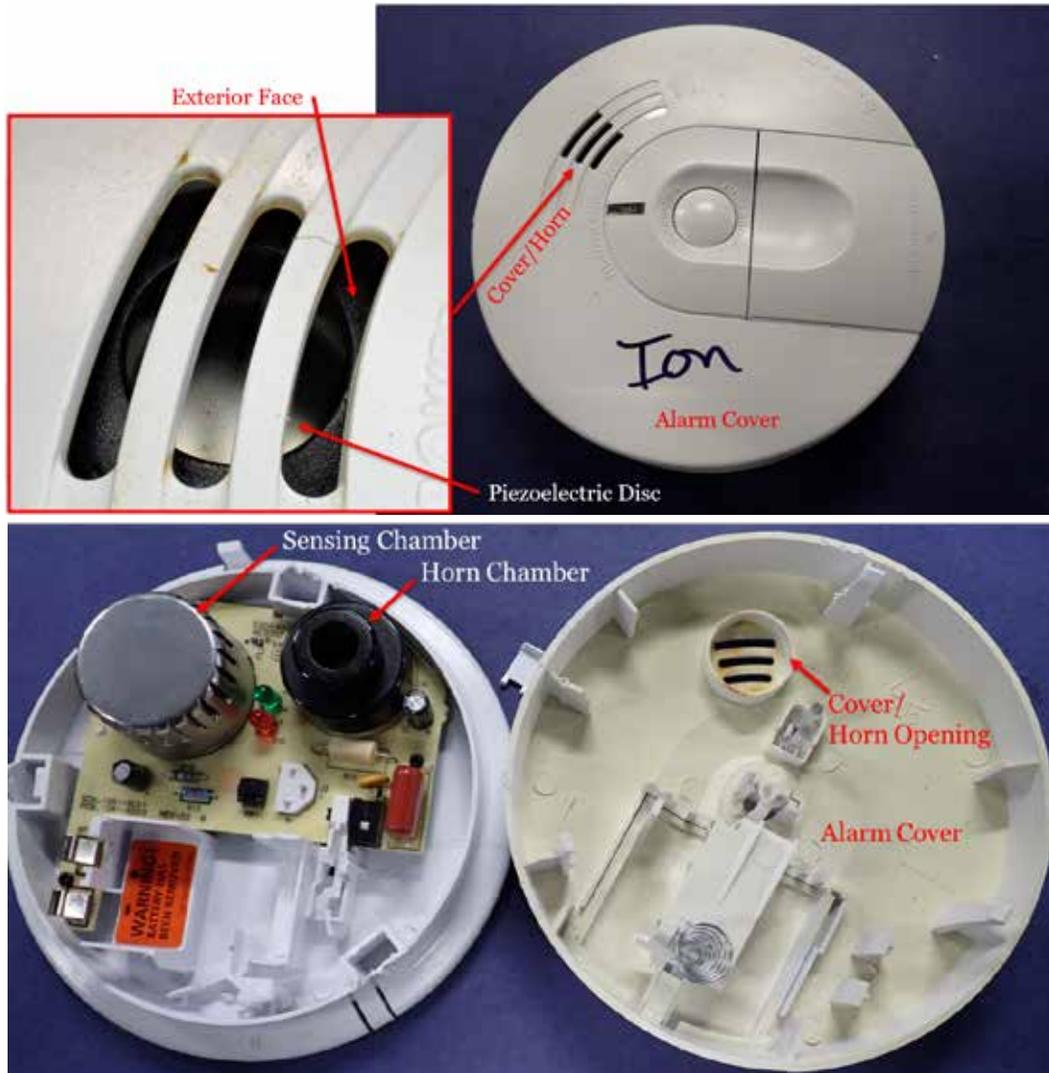
Figure 15. Example of a smoke alarm with horn chamber intimate with alarm cover opening. Note the proximity of the horn chamber opening to the alarm cover opening, and how the horn chamber extrusion fits into the inset on the alarm cover.
