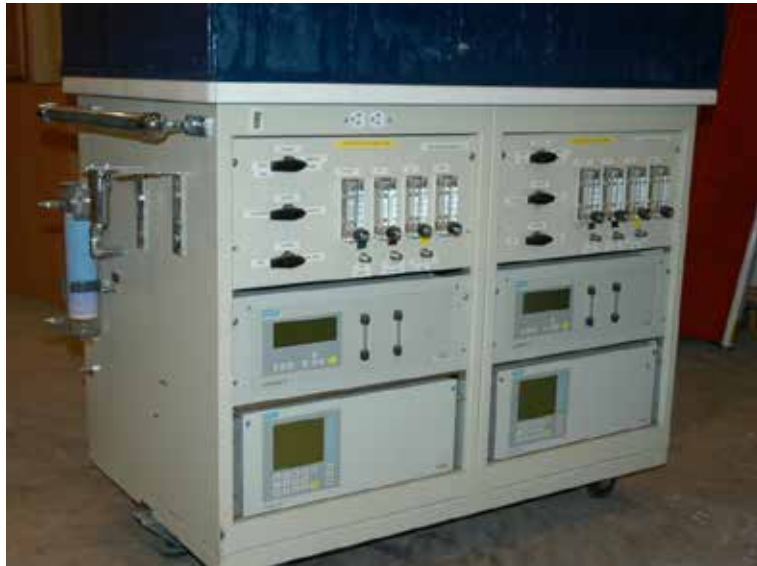
Figure 2. Cart housing of Siemens Oxymat 61 Analyzer
