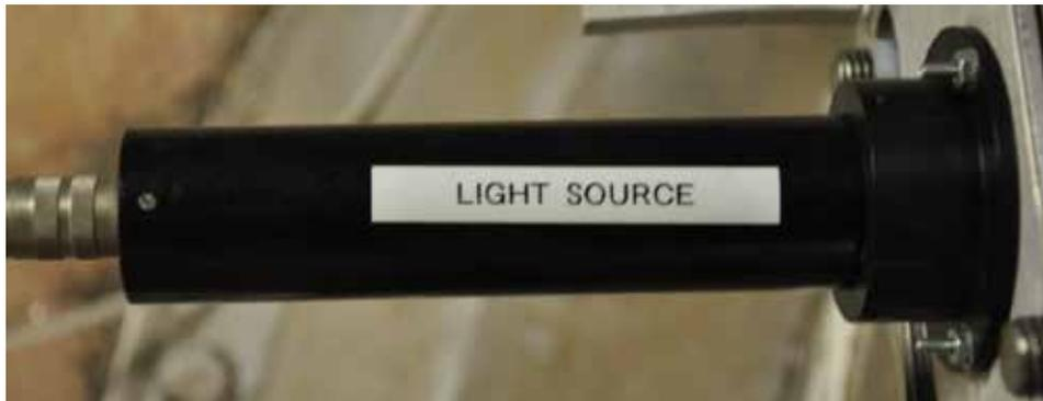
**Figure 9: Source module for white light ODM**
