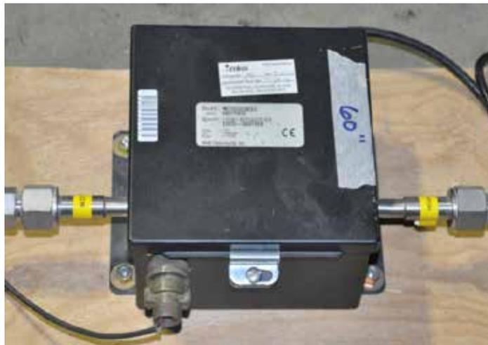
**Figure 4: MKS Type 220DD Differential Pressure Manometer**
