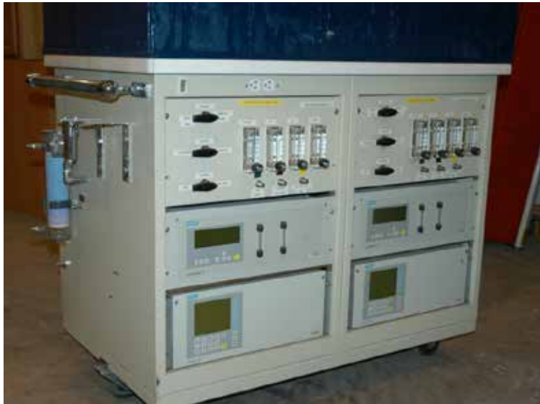
Figure 2. Cart housing of Siemens Ultramat 23 Analyzer
