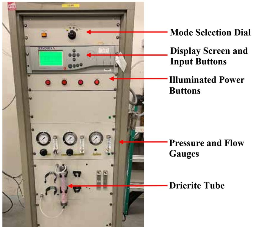
Figure 2. Analyzer Rack
