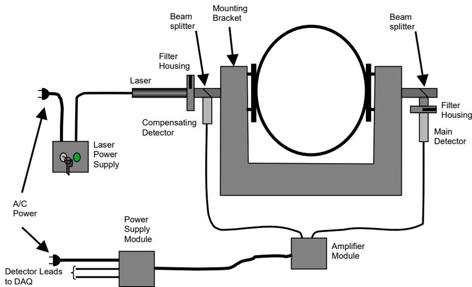
**Figure 1: Layout of laser smoke measurement equipment.**
