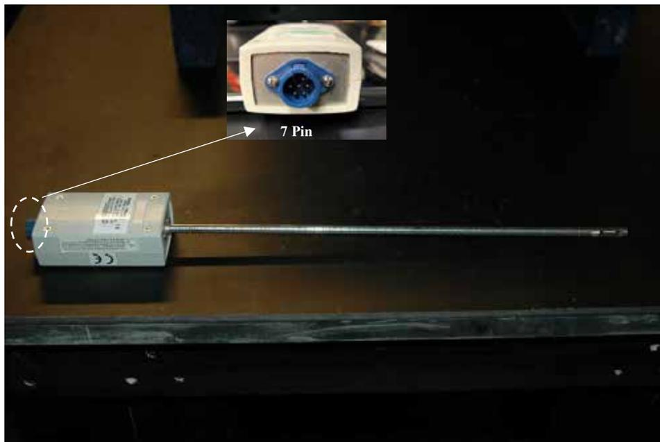
**Figure 2. FMA-901-I - Probe Attached to Electronics Box**
