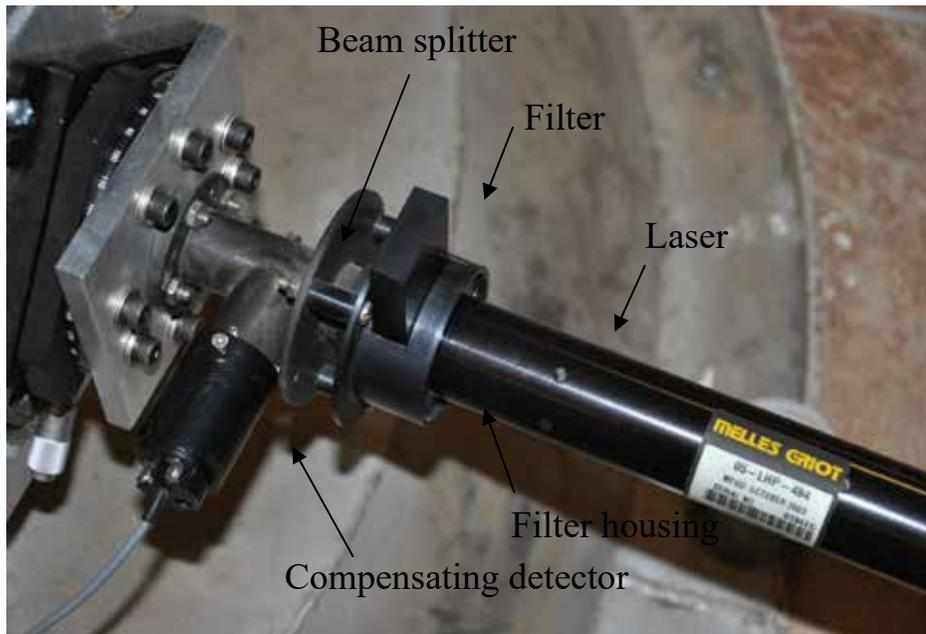
**Figure 2: Laser assembly**
