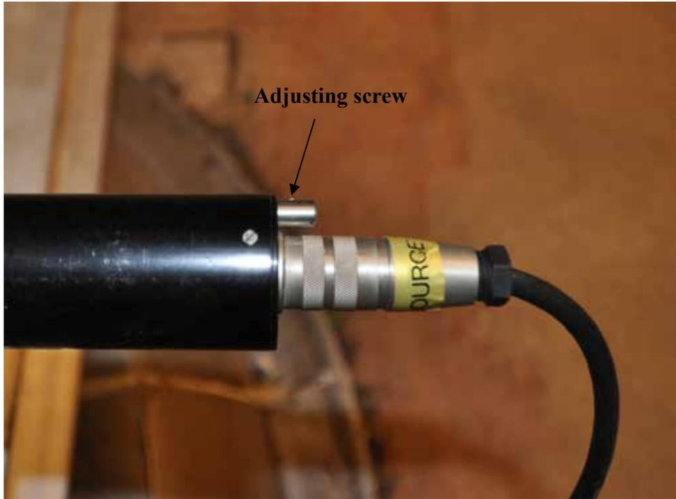
**Figure 1: Location of adjusting screw on light transmitter**
