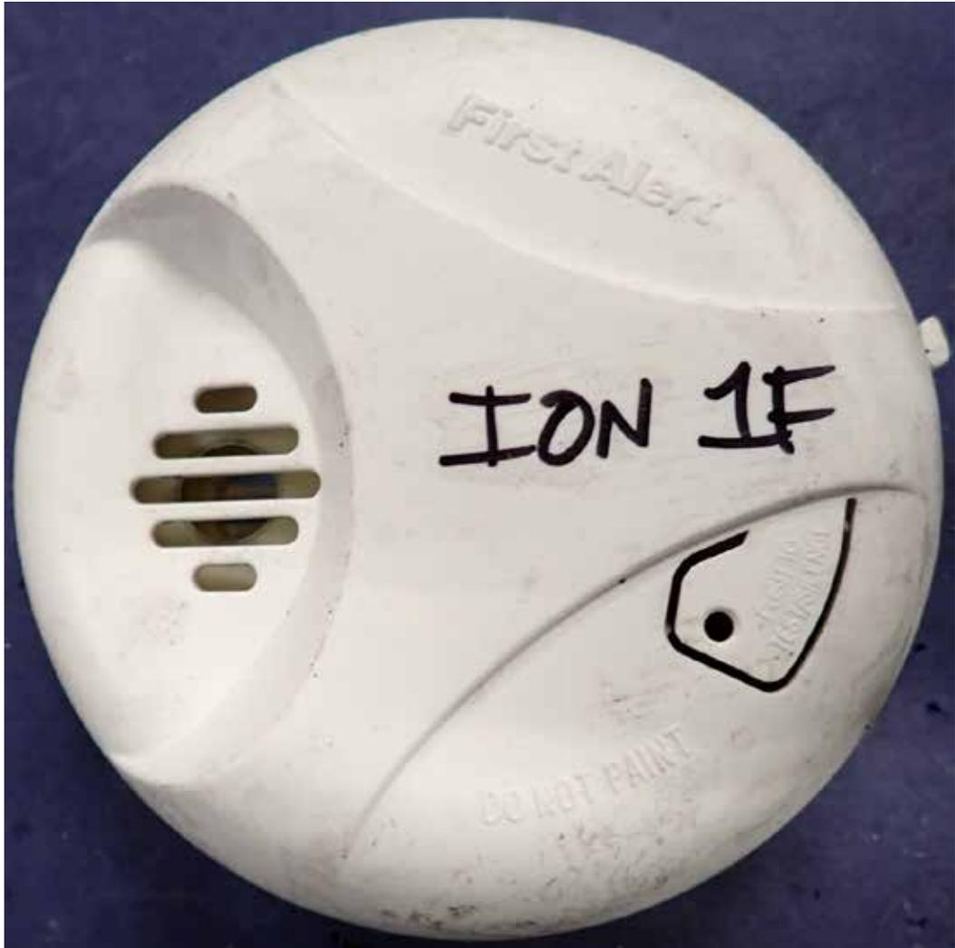
Figure 7. Example of a smoke alarm with sufficient, overall depositions of products of combustion. Note the general, relatively uniform, soot staining on the entire surface of the alarm cover.
