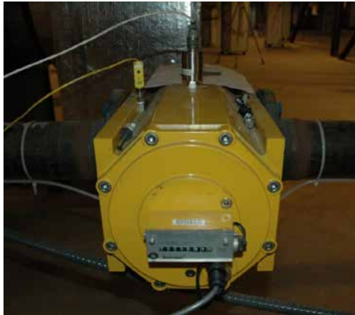
Figure 5 – Instromet IRM-A Rotary Gas Meter with mounted pressure transducer and thermocouple
