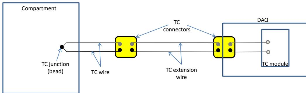
**Figure 1. Thermocouple measurement system**
