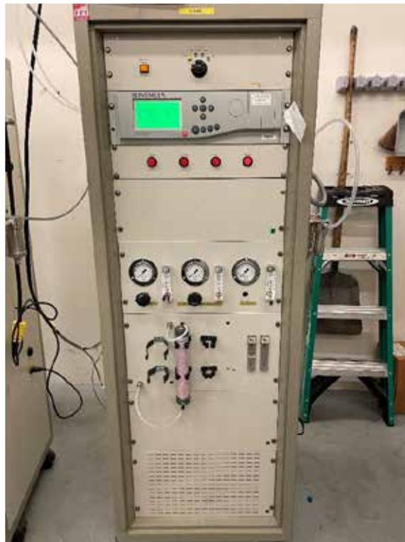
**Figure 1. Servomex 4100 Gas Analysis Rack**
