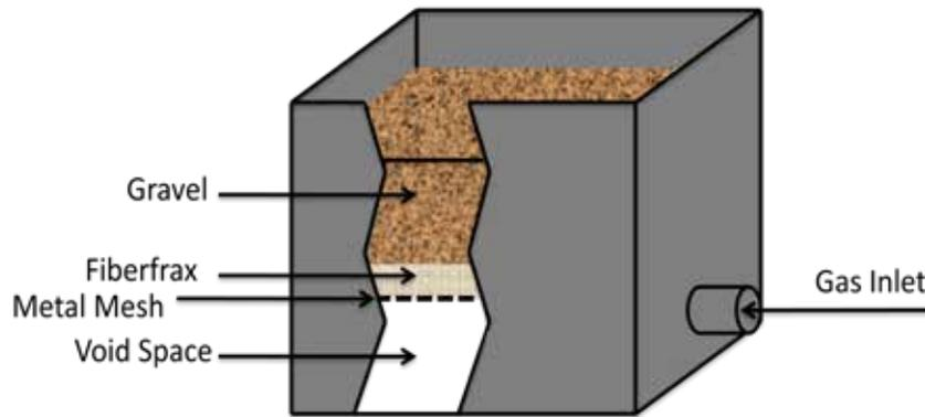
**Figure 4 – Diagram of a Typical Sand Burner**
