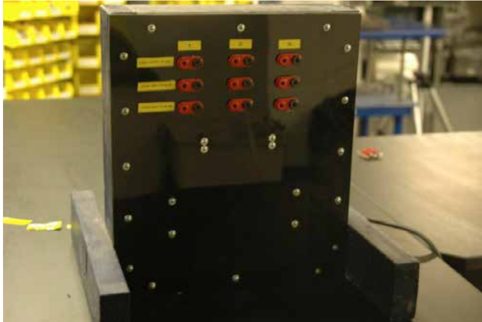
Figure 5. DAQ/power supply patch panel for hot wire anemometers
