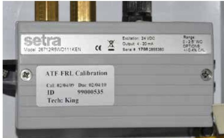
**Figure 5: Setra Model 267 Differential Pressure Transducer**
