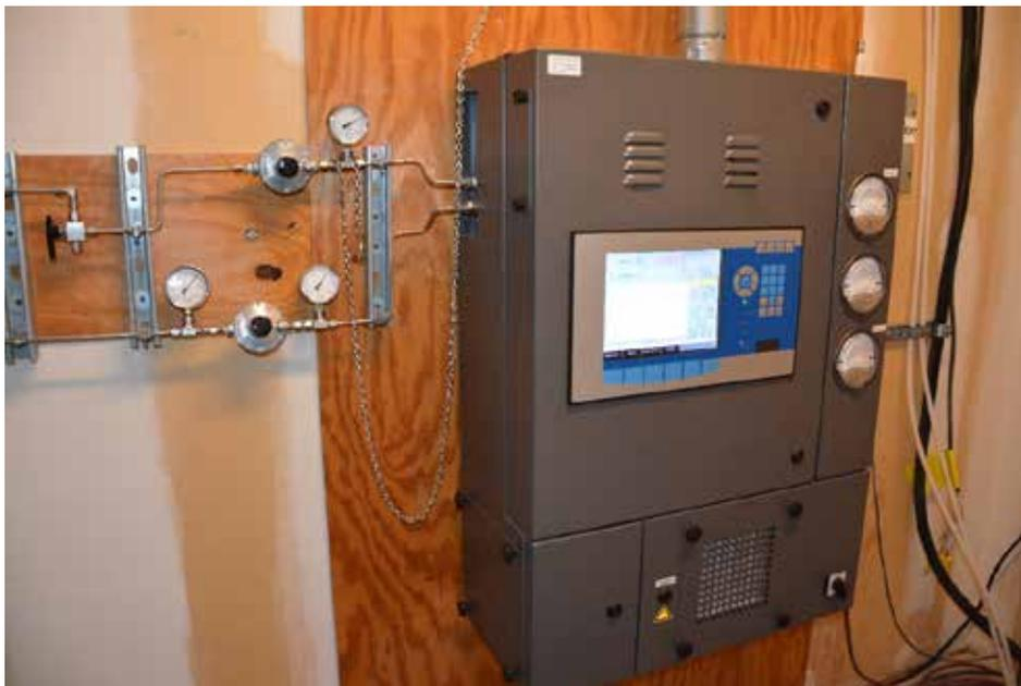
**Figure 1. Combustion Calorimeter.**
