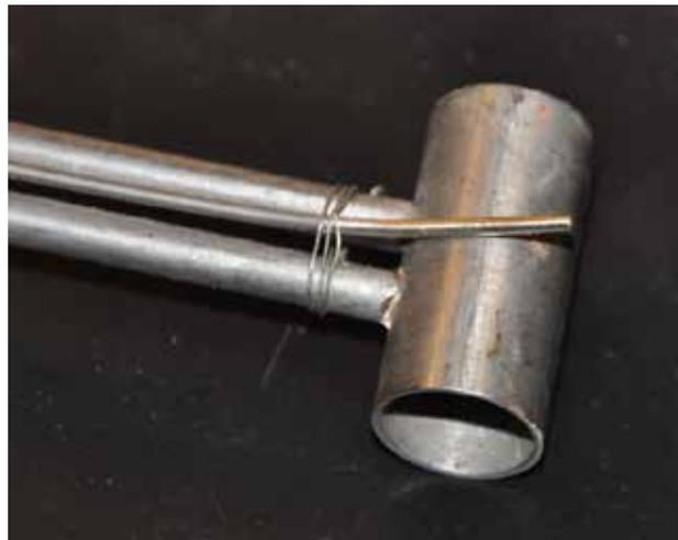
**Figure 3: Shielded thermocouple mounted to a bi-directional probe**
