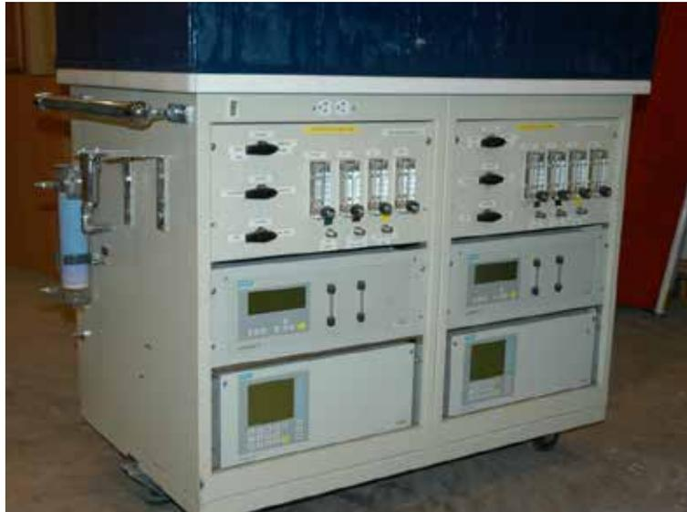
**Figure 2. Cart housing of Siemens Oxymat 61 Analyzer**
