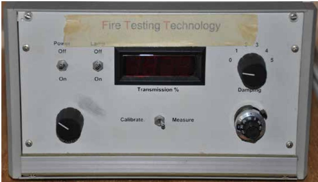
**Figure 8: White light ODM control module**
