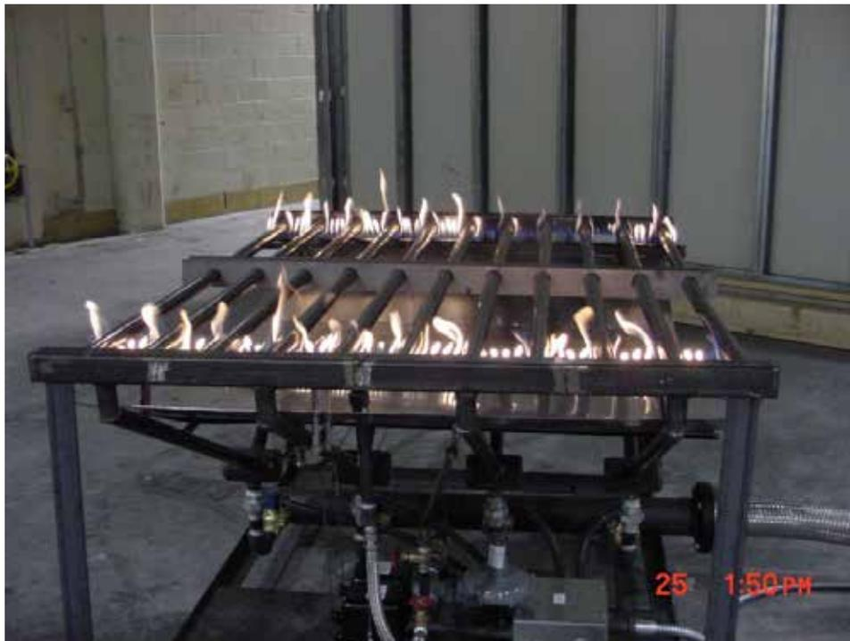
**Figure 8. Tube Burner (shown with pilot bank ignited)**
