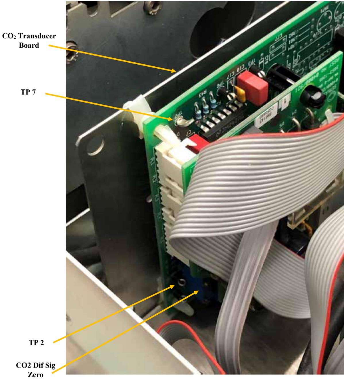
**Figure A2. CO<sub>2</sub> Transducer Board**
