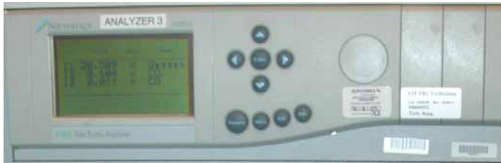
**Figure 1: Servomex 4100 Gas Purity Analyzer**
