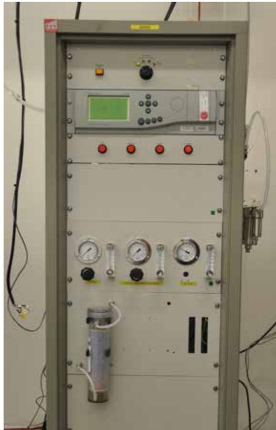
**Figure 6: Photo of the 4 MW FPC gas analysis rack**
