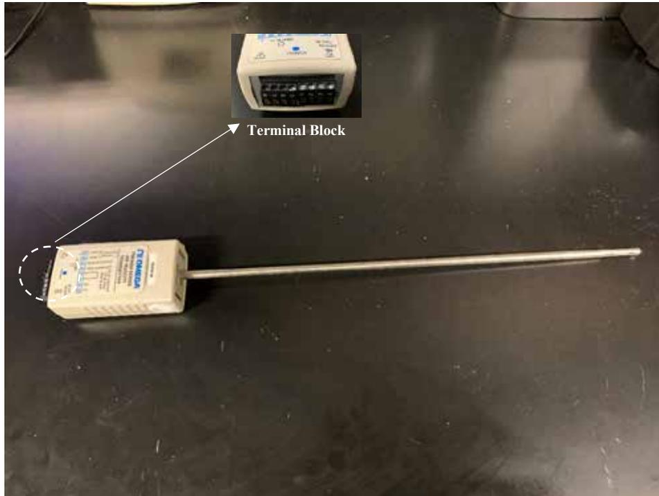
**Figure 1. FMA-900-MA - Probe Attached to Electronics Box**
