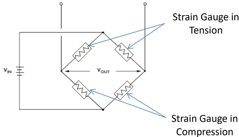
**Figure 2. Wheatstone bridge circuit with a full-bridge configuration**
