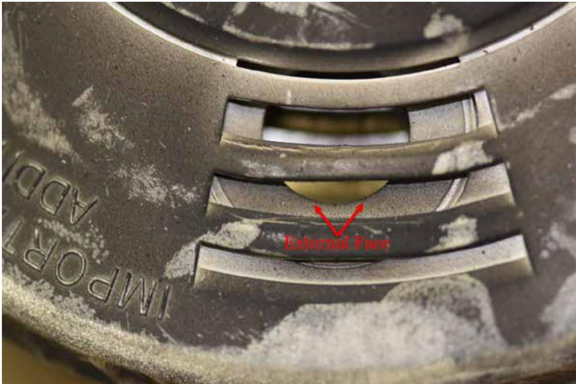
Figure 40. Example of an exposed smoke alarm without ESD on the external face of the horn chamber. Note the relatively uniform distribution of soot on all exposed surfaces.
