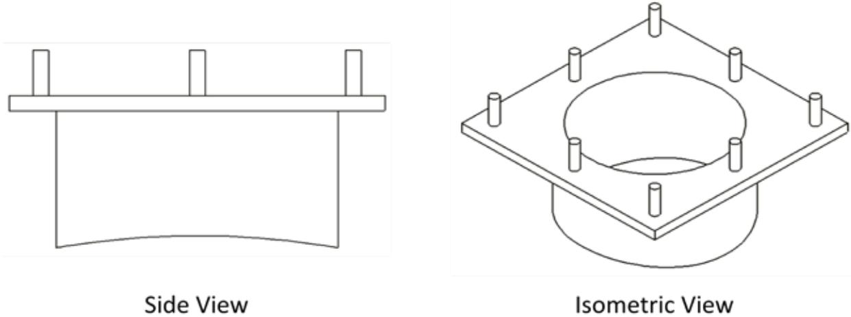
**Figure 4: The mounting bracket used to mount the probes to the exhaust duct.**
