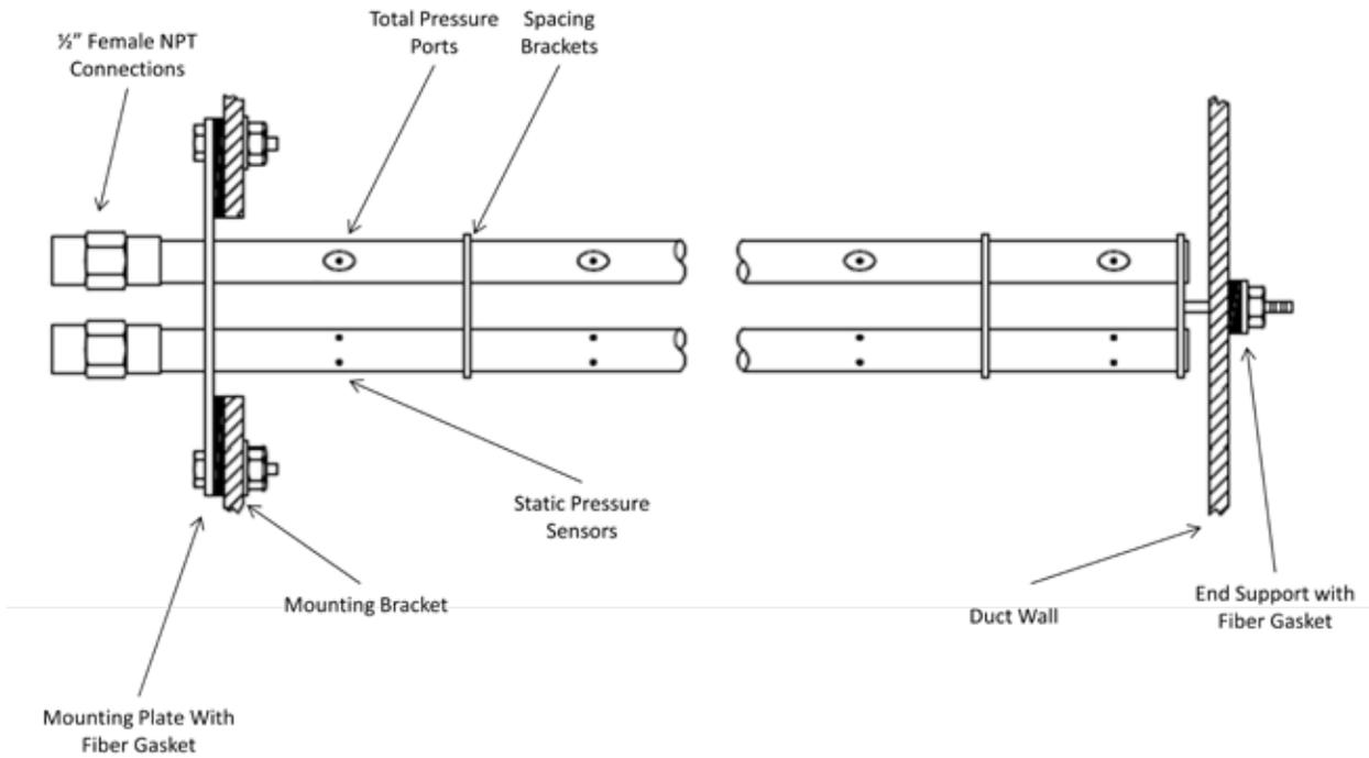
Figure 2: Schematic of the velocity traverse probes [2].
