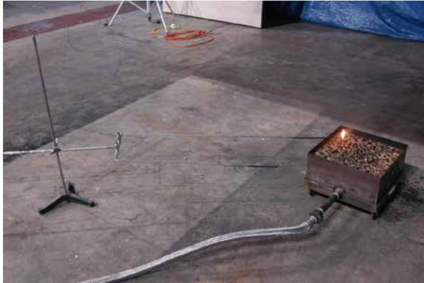
**Figure 6. Propane “Wand” Ignition Source**
