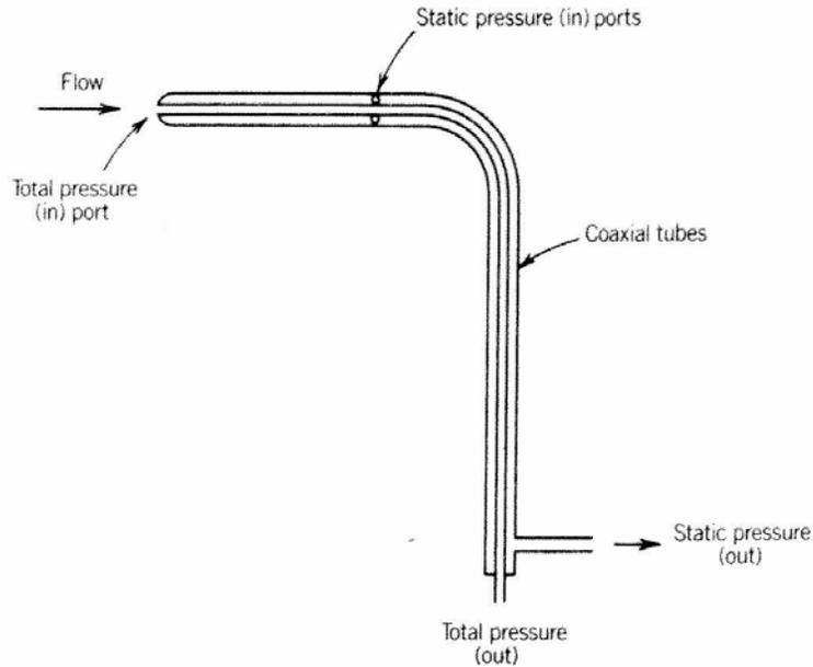
**Figure 1: Schematic of a Pitot-static probe [1]**
