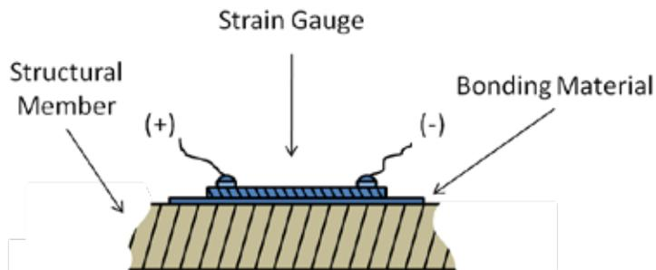
**Figure 1. Strain gauge bonded to the structural member of a load cell**
