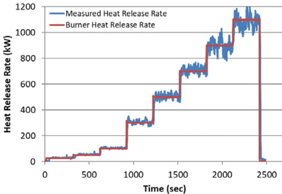
Figure 3. Measured Heat Release Rate Corrected with C-Factor
