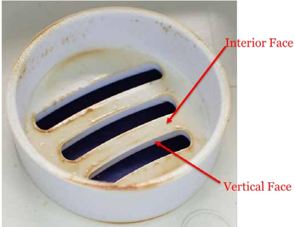
Figure 10. Example of a smoke alarm with horn chamber physically connected to the alarm cover backside the piezoelectric disc has been removed, exposing the horn chamber interior, interior and vertical faces.
