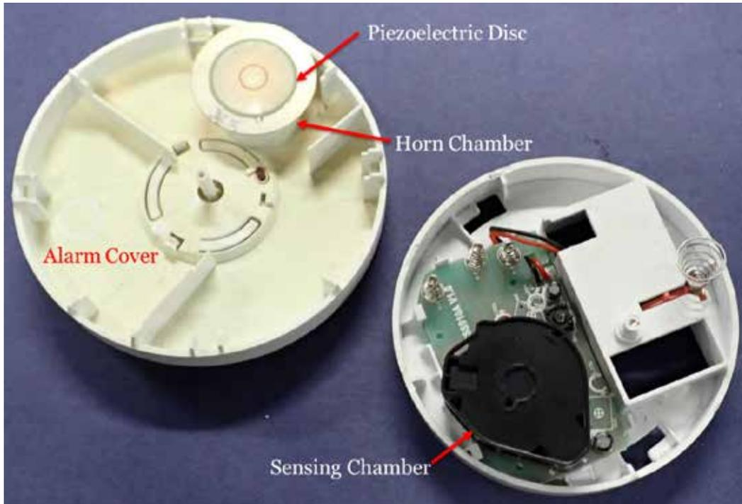
Figure 9. Example of a smoke alarm with horn chamber exterior face located on the exterior of the alarm cover. Note how the horn chamber is physically connected to the alarm cover backside (Bottom), backed by the piezoelectric disc.
