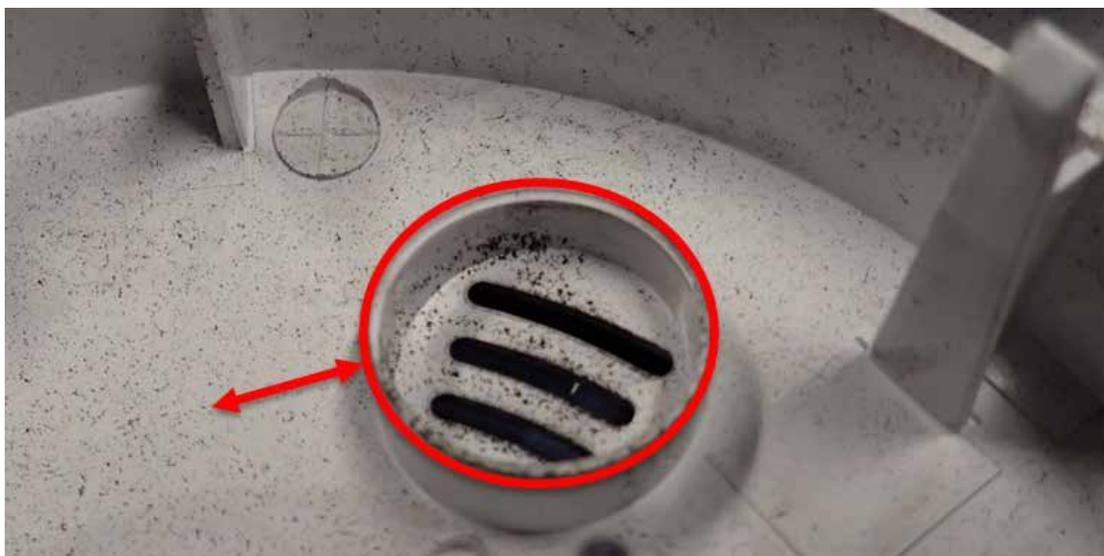
Figure 24. ESD observed within the alarm cover inset for the horn chamber. Note the differential soot deposition (more) with relative to that observed on adjacent surfaces.
