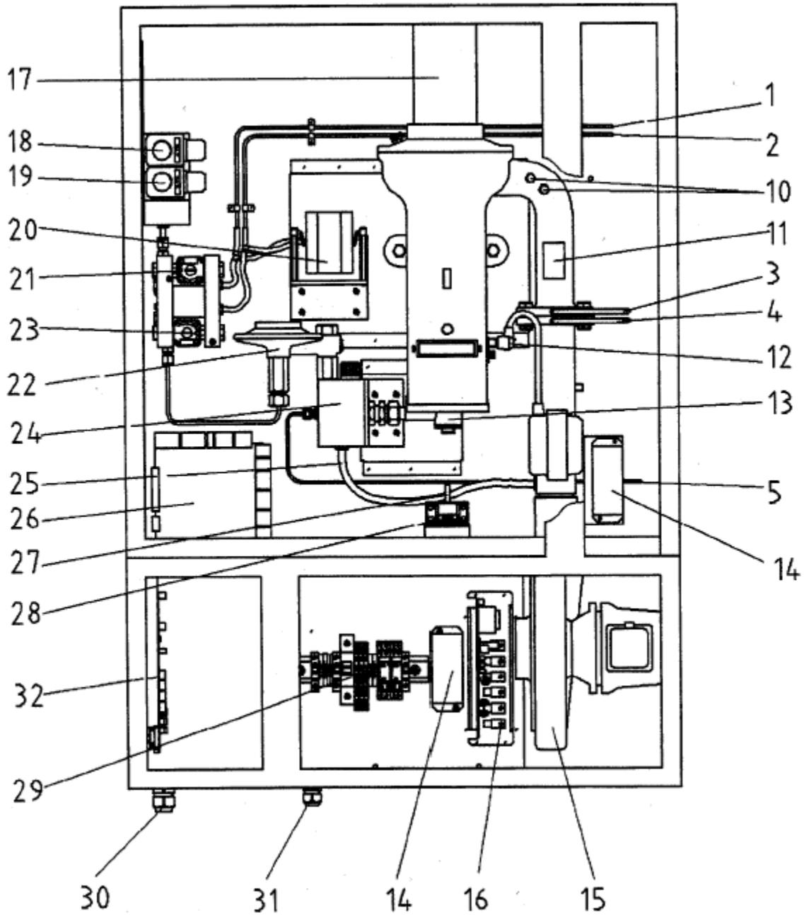
Figure 2: Inside View of CWD 2000 Combustion Calorimeter [1]
