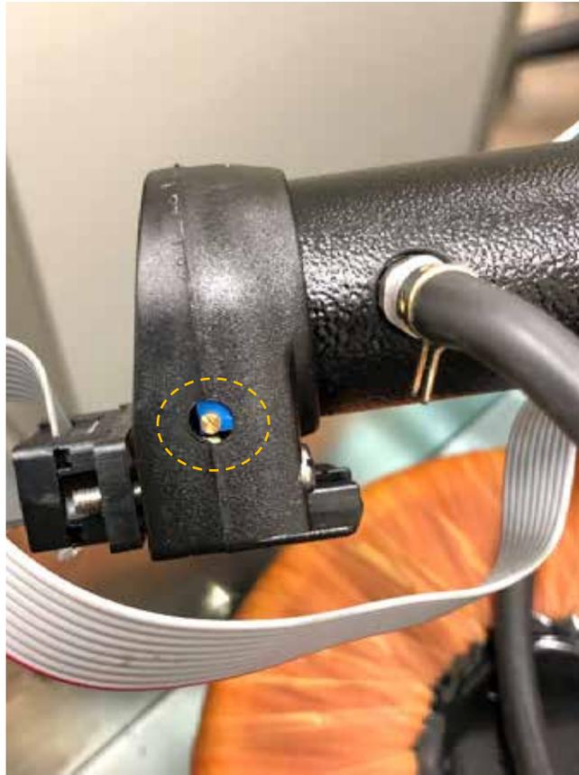
**Figure A5. CO Cell Coarse Zero Potentiometer**
