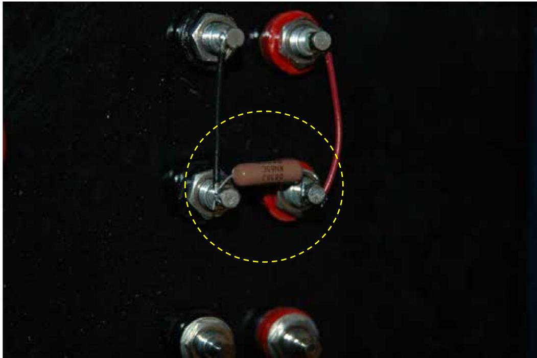
Figure 6. A 250 ohm resistors used in patch panels
