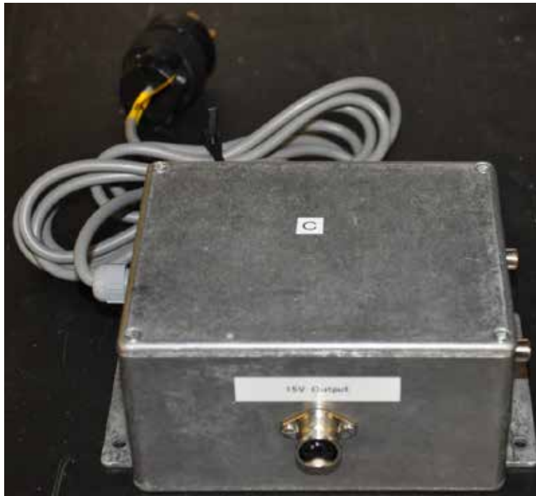
Figure 6: Laser ODM power supply module
