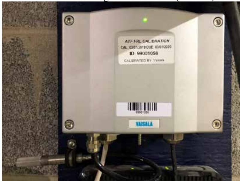
Figure 1. Vaisala PTU300 transmitter and PTU303 probe
