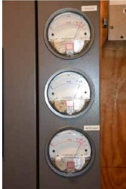
**Figure 5. Combustion Calorimeter Pressure Gauges.**
