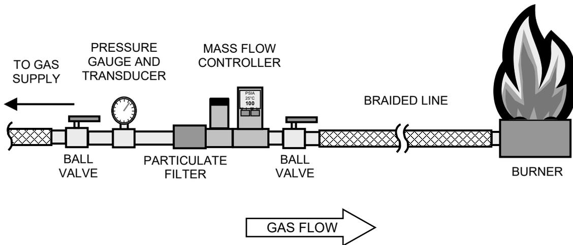
Figure 1. Sand burner and gas cart setup
