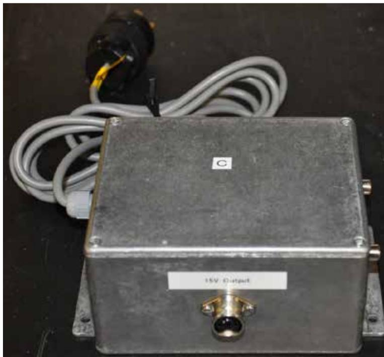
**Figure 6: Laser ODM power supply module**
