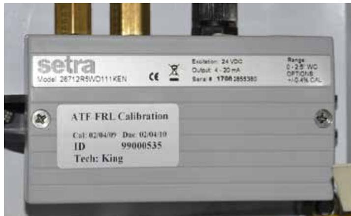
**Figure 6: Setra Model 267 Differential Pressure Transducer**
