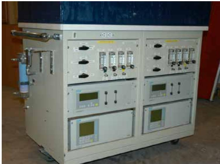
**Figure 2. Cart housing of Siemens Ultramat 23 Analyzer**
