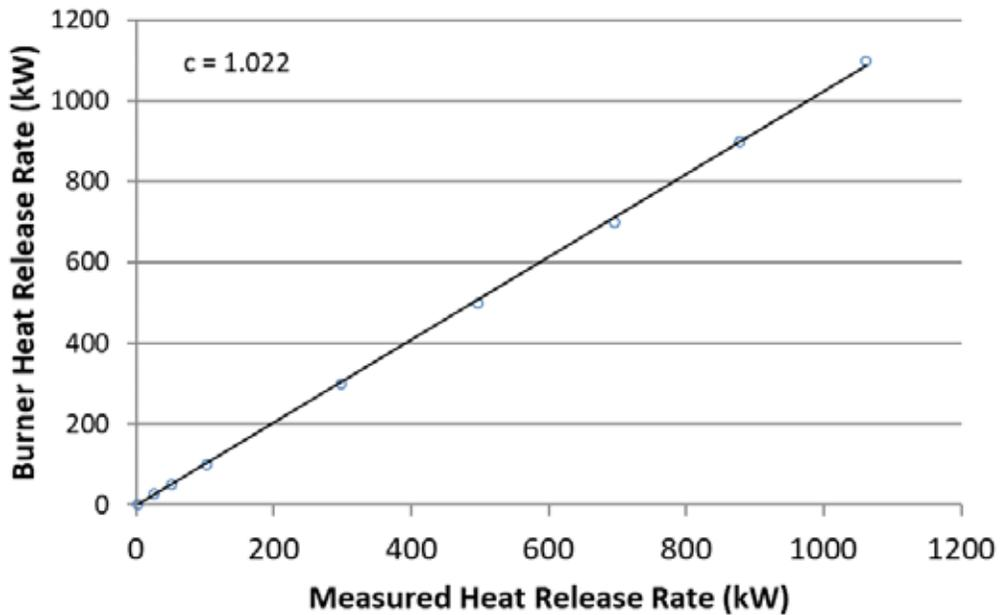
Figure 2. Example of a Nine-Point Burner C-Factor Determination
