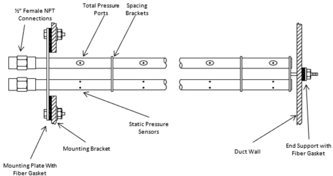
Figure 8: Schematic of the velocity traverse probes [10].
