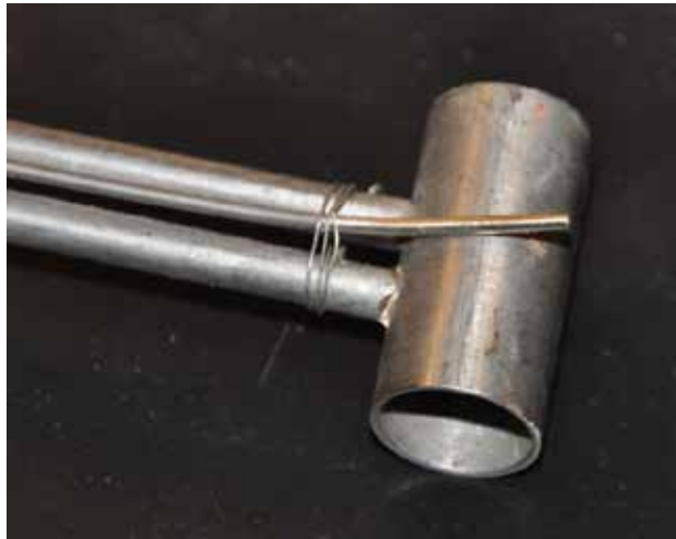
Figure 3: Shielded thermocouple mounted to a bi-directional probe
