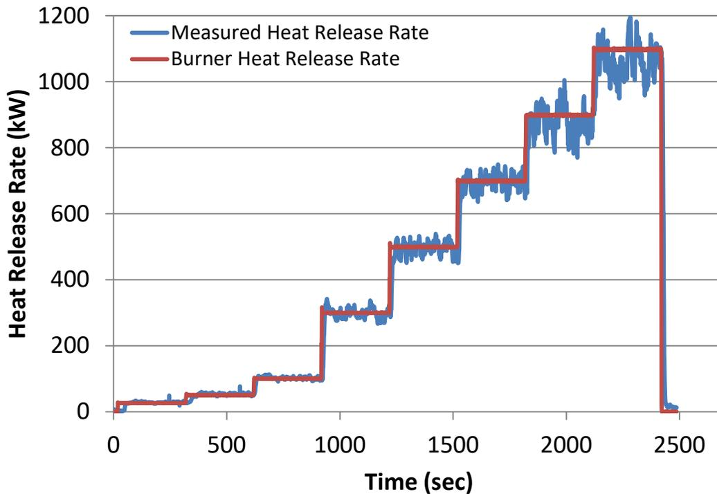
Figure 1. Example of a Nine-Point Burner Calibration Experiment
