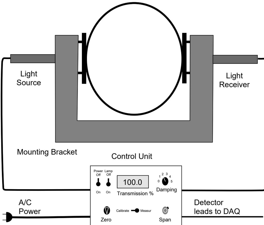
**Figure 7: Layout of white light smoke measurement equipment.**
