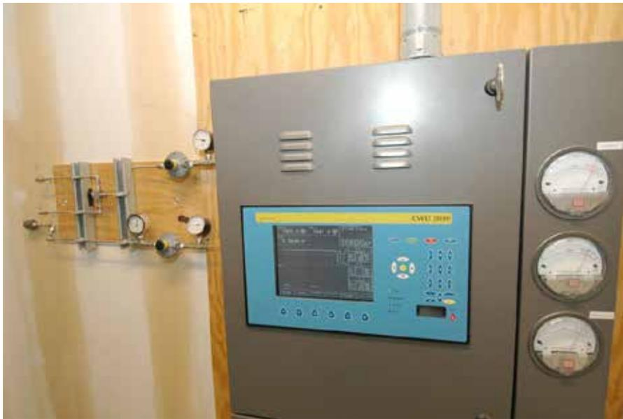
**Figure 1: Combustion Calorimeter Mounted to Wall in 1 Megawatt Shed**
